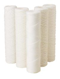
Pentair<sup>‡</sup> Pentek<sup>‡</sup> WP Series Cartridges are manufactured from a durable polypropylene string that is wound around a rigid polypropylene core. They are premium string wound solution to reduce fine sediment, including sand, silt, rust and scale particles.
