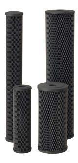
Pentair<sup>‡</sup> Pentek<sup>‡</sup> NCP Series Cartridges are constructed from a carbonimpregnated non-cellulose media. They offer sediment filtration, as well as taste, odor and chlorine taste & odor reduction in one cartridge. Unlike cellulose cartridges, NCP Series Cartridges can be used for municipal and non-chlorinated water applications.
